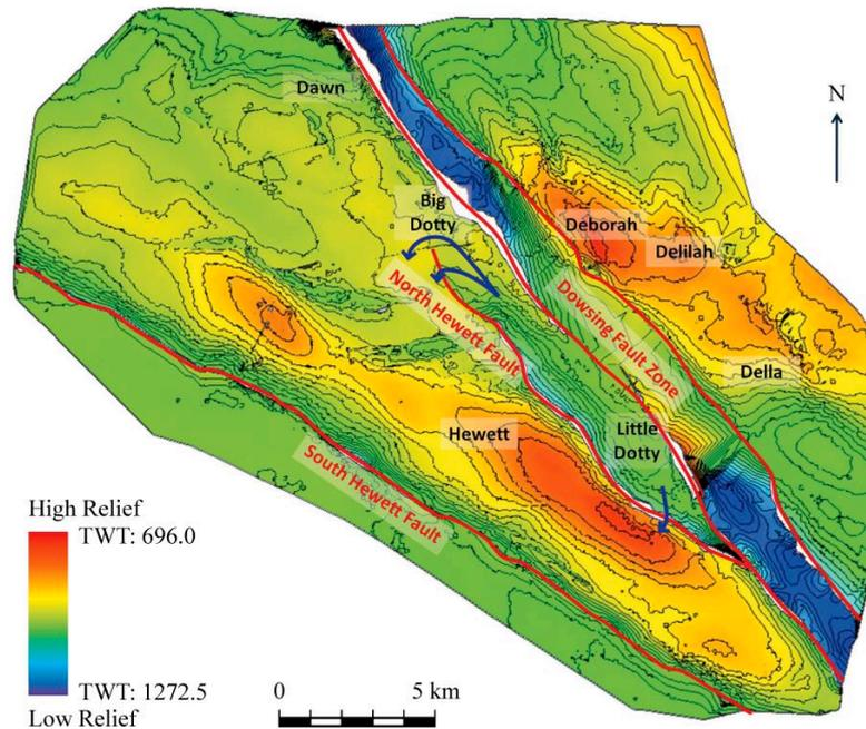
**Figure 2** Annotated time structure map of the top Bunter Sandstone Formation within the Hewett Unit. Potential pressure communication pathways, via the regional Bunter aquifer, are illustrated as dark blue arrows. Interpreted in T7
