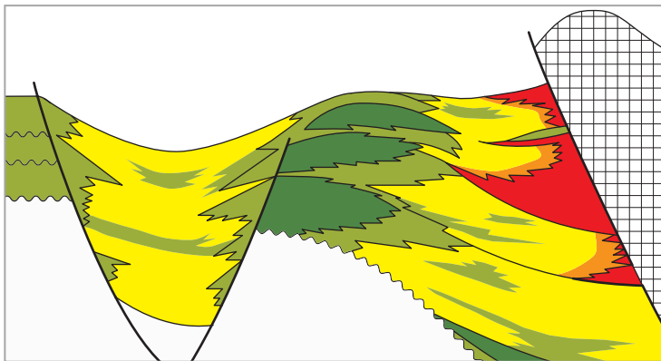
Generalised cross-section coloured by fracture quality showing the lateral variation in predicted quality.
