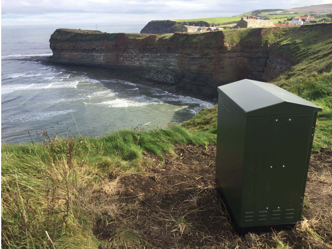
Figure 2. Deployment of an autonomous laser scanner housed in custom metal container.
