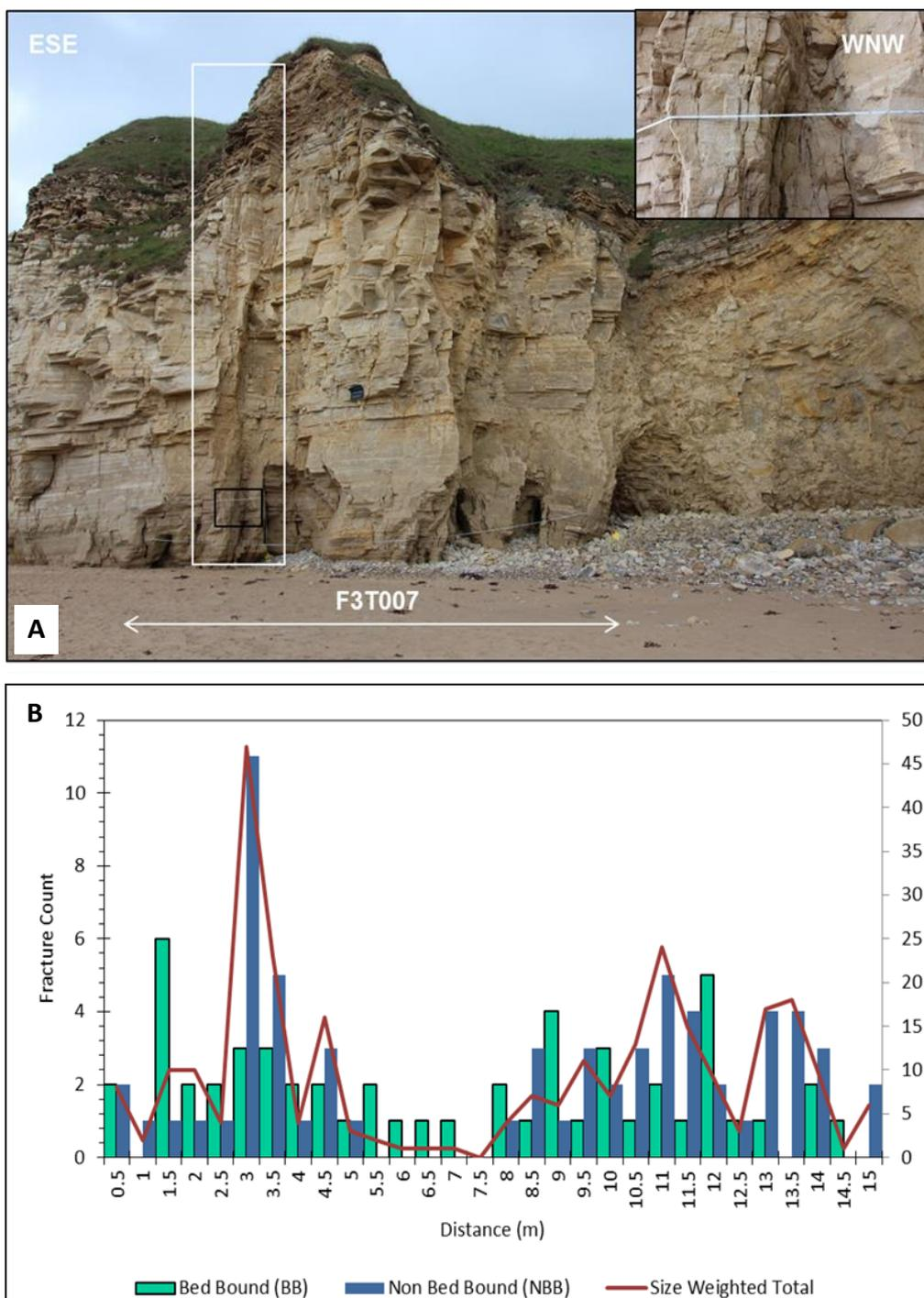
Fig.2 Fracture corridor within the Roker slope facies. **A** white box shows area of vertically persistent fractures. Black box shows the location of the inset image. **B** Fracture density per 0.5 m bin (along transect 'F3T007'). A peak in intensity of non-bed-bound fractures occurs at the point at which the inferred fracture corridor intersects the transect at 3 m.
