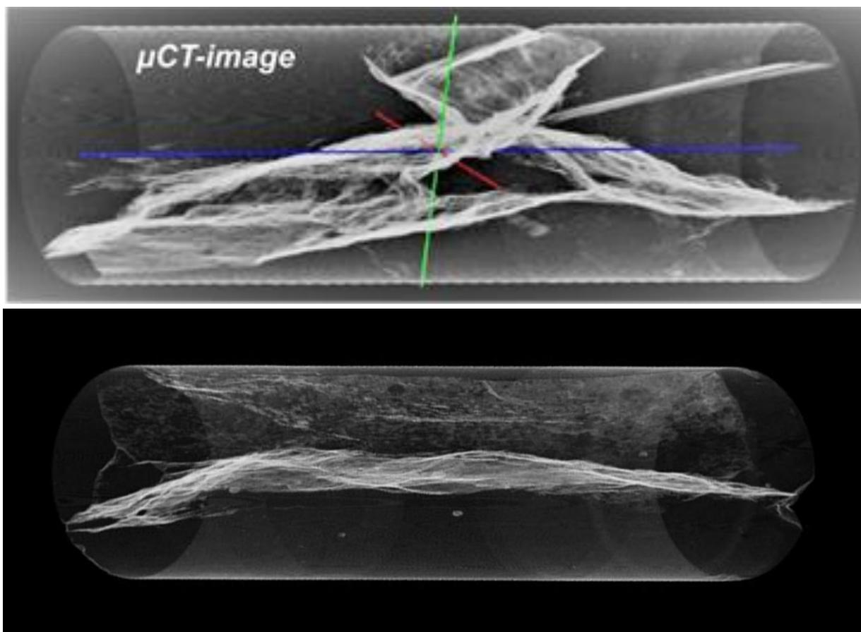
**Figure 2** Examples of high resolution micro-CT images from the examined core plugs, showing the detailed geometry of overlapping microfractures. Diameter of core plugs = 3.6cm
