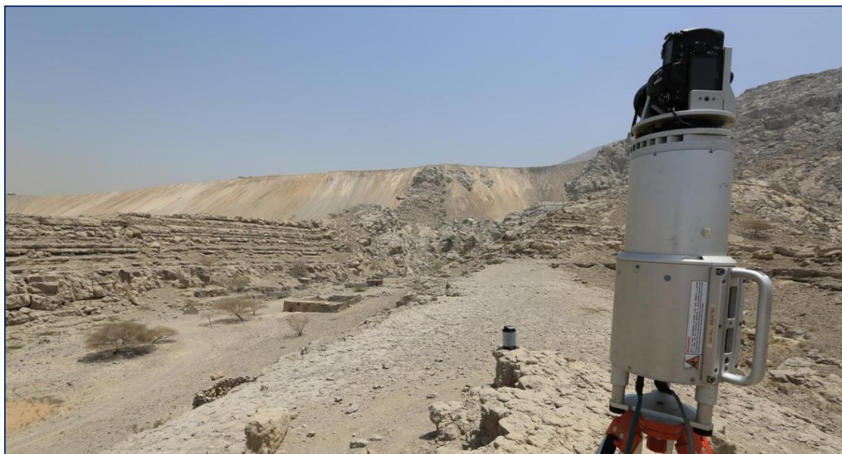
**Figure 1** Lidar scanning of Wasia and Thamama carbonates at Ras Al-Khaimah.
