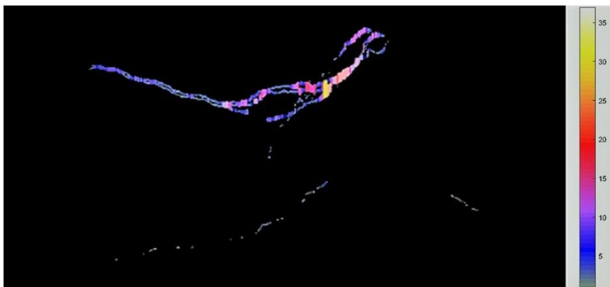
**Figure 3** Aperture variation along a slice of a mCT-image (coloured scale in voxels: 1 voxel =  $40.3\mu\text{m}$ ).
